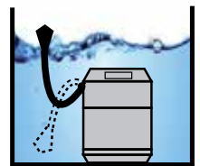
Direct connection to pump
